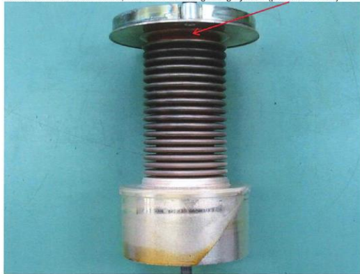
Picture 3: variable electrode, with bellows and guiding system (position of leak)
