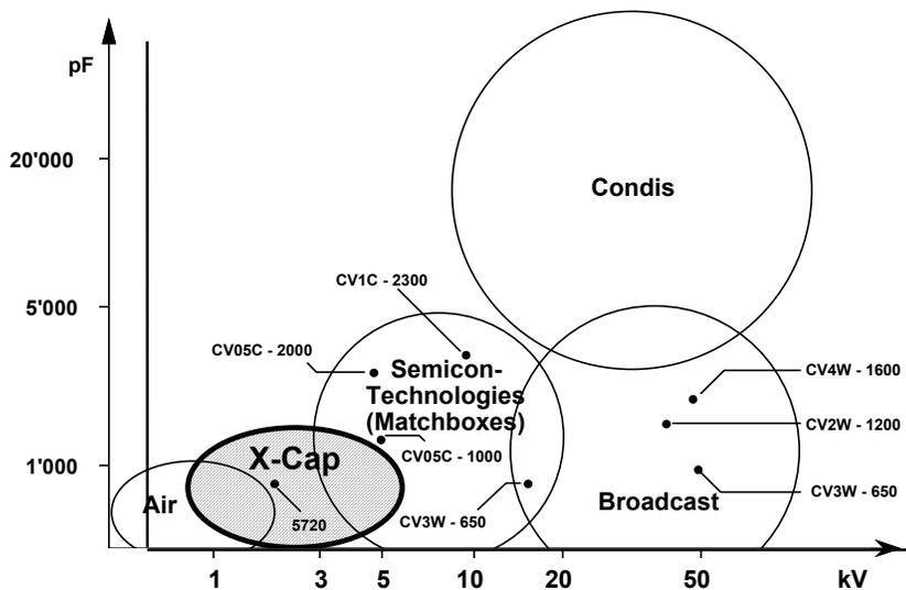
The application field of X-CAP™ is where today standard air capacitors are used but assuring better performance. Due to the hermetically closed design, it is particularly suitable for rugged and dirty environments (dust, oil, vapors ... ). This device will work for years without the need of any maintenance work. It is obvious, that the X-CAP™ can fill the gap between the air and vacuum capacitor and even the lower end of the vacuum capacitor applications.
