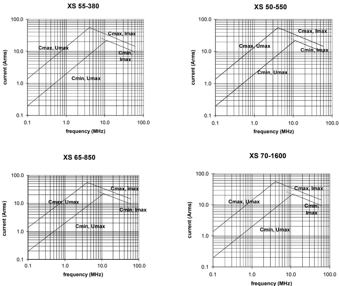
Above figures were measured without any forced cooling. To increase current capabilities at higher frequencies it is suggested to cool the connecting plate of the X-CAP™ by adding a cooling flange for forced air- or water cooling. It is also very helpful to cool the capacitor housing by means of an air blower.
