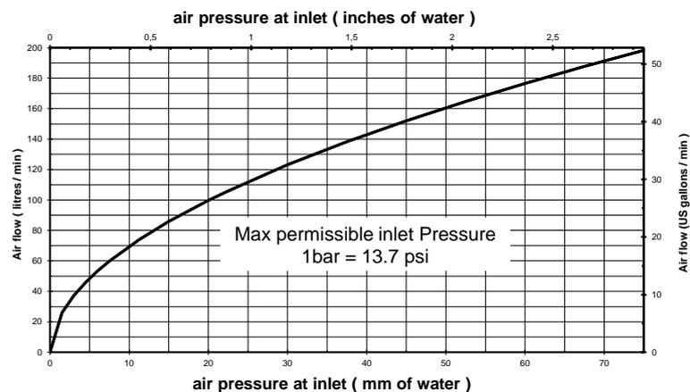
**Fig. 8:** Air flow vs. air pressure (typical)
