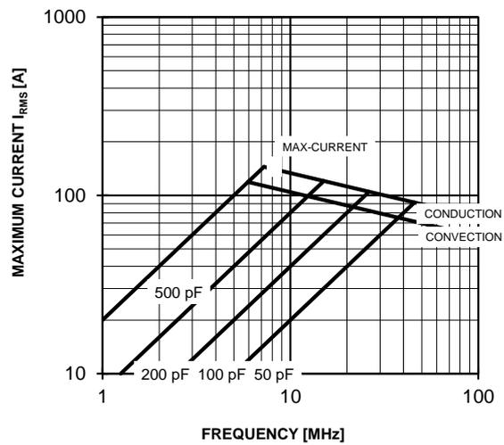
**Fig 6:** Typical current vs. frequency and capacitance
