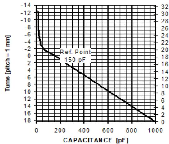
Fig 3: Typical turns vs. capacity
