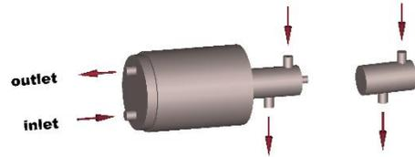
**Fig. 11:** Vacuum capacitors requiring 22 l/minute minimum, usually 25 l/minute
