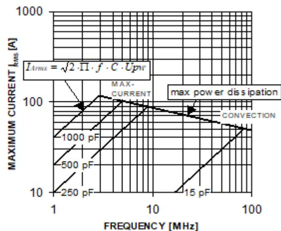
**Fig. 2:** Typical current vs. frequency and capacitance
