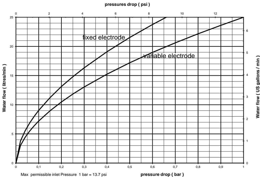
**Fig. 13:** Pressure drop across capacitor vs. water flow (typical)
