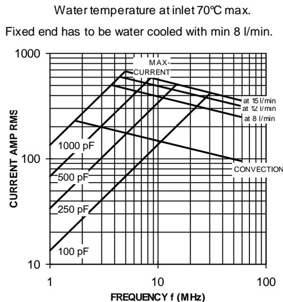
**Fig. 9:** Typical current vs. frequency and capacitance
