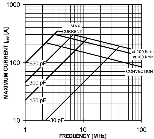
**Fig 7:** Typical current vs. Frequency and capacitance
