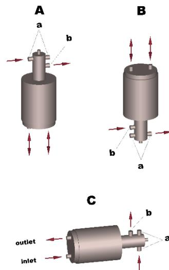
**Fig. 10:** Vacuum capacitors with water flow up to 15 l/minute
