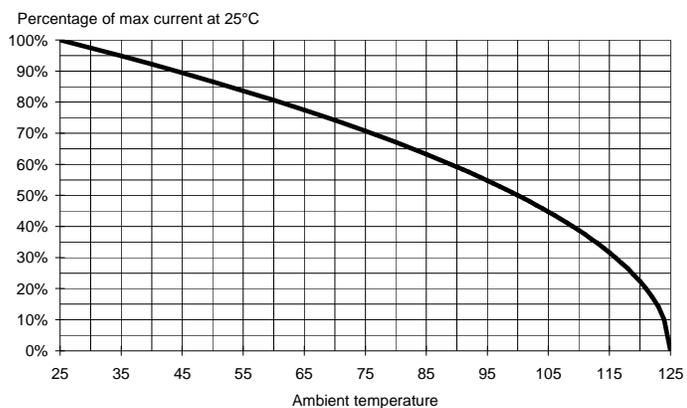
**Fig.5:** Derating RF current in percent of maximum permissible current at 25° C ambient temperature
