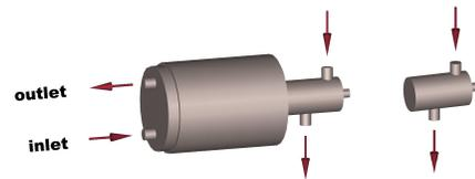
**Fig. 10:** Vacuum capacitors requiring 22 l/minute minimum, usually 25 l/minute
