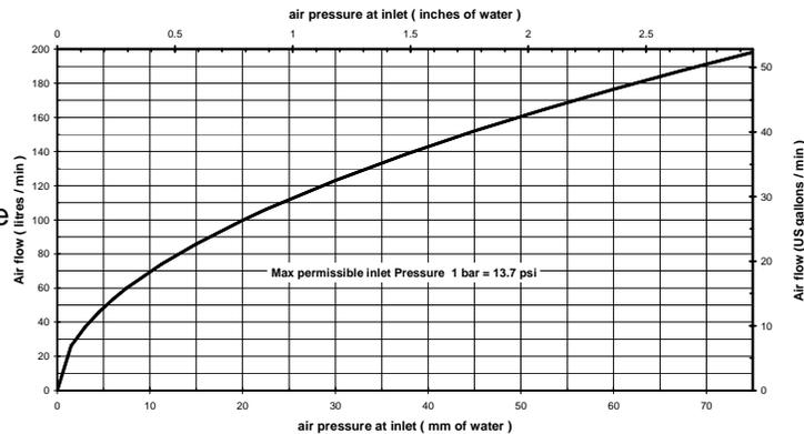
**Fig. 7:** Air flow vs. air pressure (typical)
