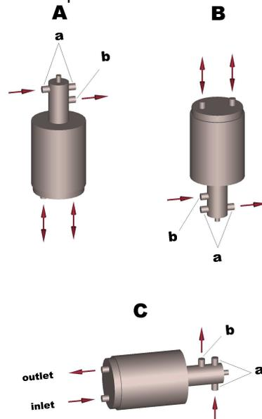
Fitting "a" is located on some water-cooled types on the same side as fitting "b". The formation of trapped bubbles along the bellows or in its immediate vicinity is avoided for mounting positions A and B and will then flow in direction as indicated. It is minimized in position C, such that trapped bubbles cannot cause fatal damage due to lack of cooling under normal operating conditions.
