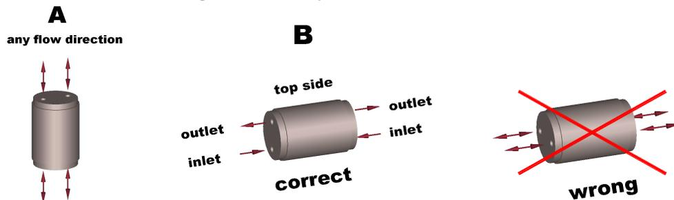
**Fig. 11:** Water connections for water-cooled fixed capacitors
