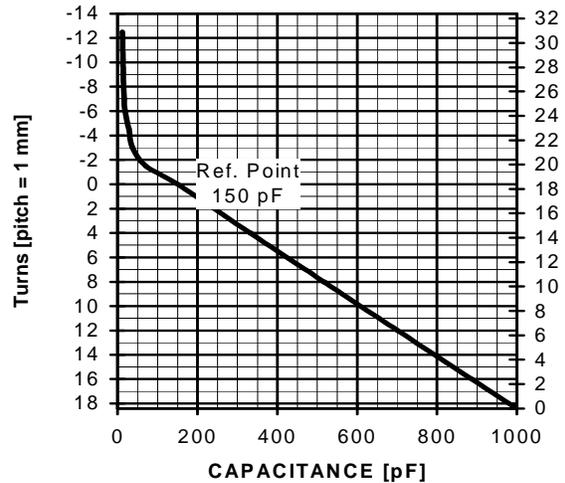
**Fig. 3:** Typical turns vs. capacity
