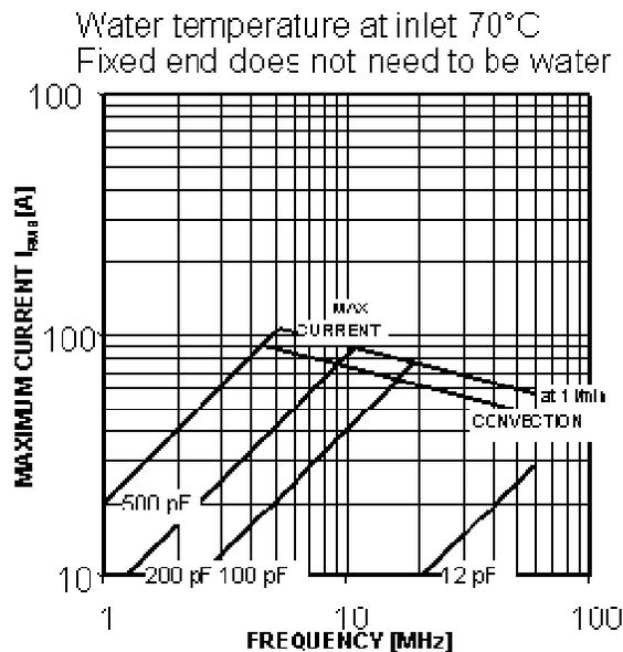
Fig. 13: Current curve CVMI-500AW/15-AAC-M
