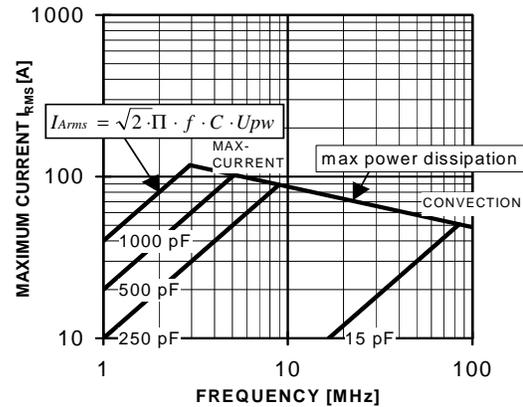
**Fig. 2:** Typical current vs. frequency and capacitance
